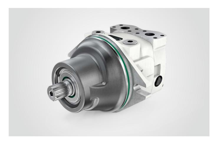
The Liebherr axial piston motor FMF series is developed for the open and closed circuit in swash plate design. The fixed plug-in motors are available in finely graded nominal sizes ranging from 25 to 250 cm<sup>3</sup>. The nominal pressure is 350/420 bar and maximum pressure 380/450 bar, depending on its size.
