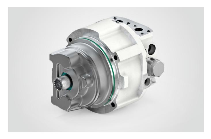
The Liebherr axial piston motor CMVE series is developed for the open circuit in swash plate design. The variable plugin motors are available in nominal sizes ranging from 85 to 165 cm<sup>3</sup>. The nominal pressure is 380 bar and maximum pressure 400 bar.
