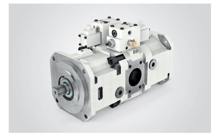
The Liebherr axial piston pump DPVD series is developed for the open circuit in swash plate design. The variable pumps are available in nominal sizes 108-108 and 165-165 cm<sup>3</sup>. The nominal pressure is 400 bar and maximum pressure 450 bar.
