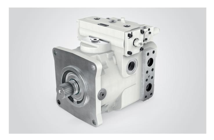
The Liebherr axial piston pump DPVG series is developed for the closed circuit in swash plate design. The variable pumps are available in nominal sizes ranging from 85 to 280 cm<sup>3</sup>. The nominal pressure is 450 bar and maximum pressure 500 bar.
