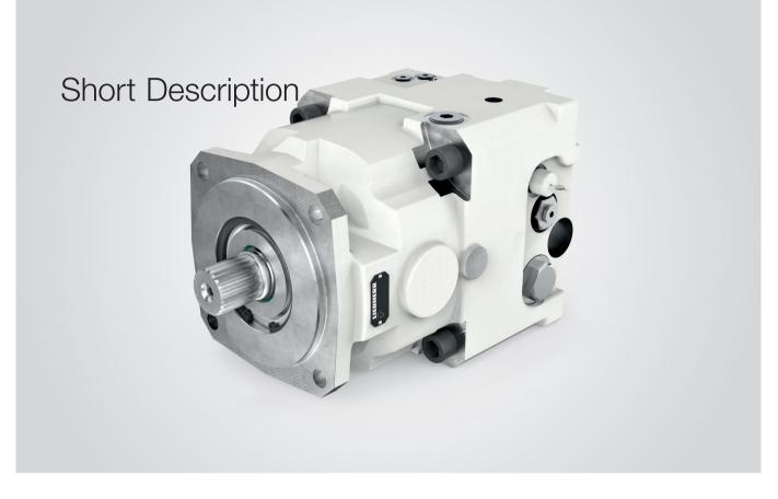
The Liebherr axial piston motor DMVA series is developed for the open and closed circuit in swash plate design. The variable flange motors are available in nominal sizes ranging from 108 to 370 cm<sup>3</sup>. The nominal pressure is 450 bar and maximum pressure 500 bar. For size 370, the nominal pressure is 400 bar and maximum pressure 450 bar.
